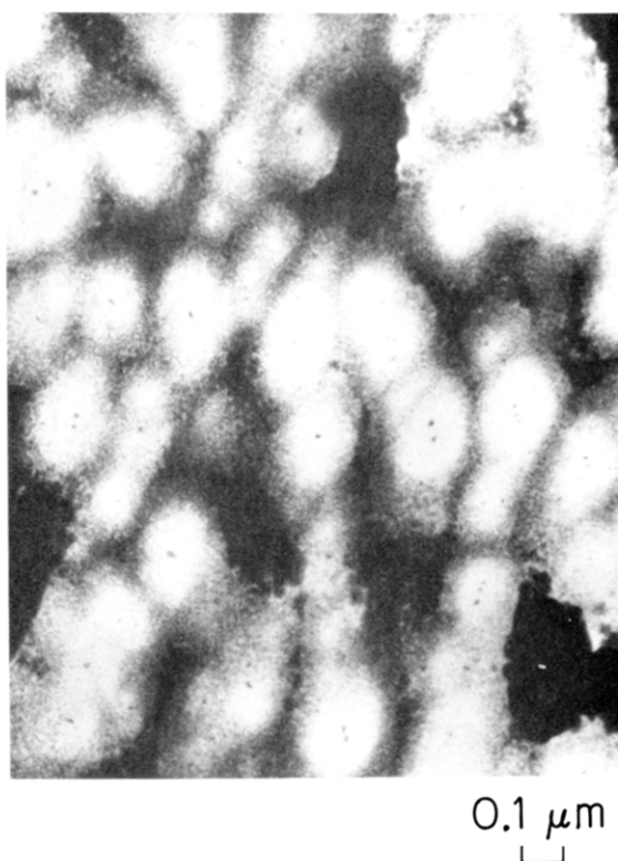
Figure 6. TEM photograph of sample C prepared with the Ti(OR) 0.5 Cl 3.5 /MgCl 2 -supported catalyst system.
